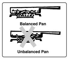
**Use balanced pans** that sit level on the burner grate without tilting from the weight of the handle.
